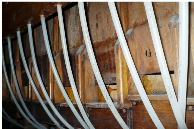
Tubular-pneumatic tubes for upper Bourdon notes
