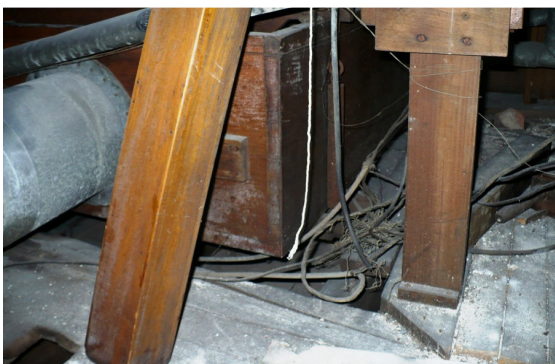
Gt-Ch-Ped reservoir wind line, offset chest for Gt. Melodia on right, with pipe in foreground
