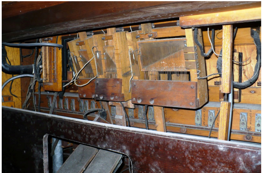
Just below the keyboards: coupler actions and combination actions. The magnets are coupler and stop primaries.
